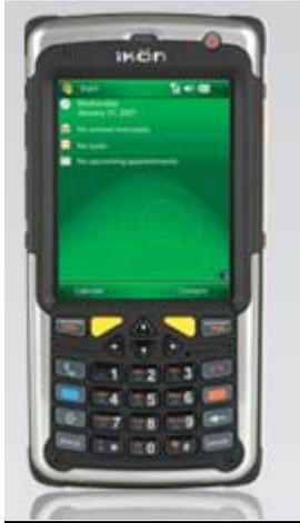
The Ikon In-cab unit has been operated by Bakers Waste on an FEL Bin round and skip round for the purposes of the trial. The round data is held in the ISYS waste management system and the movements are sent to the Ikon handheld which is situated in the drivers cab.
